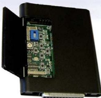
FlashBack-2 Motion Detector showing set up buttons and switches
