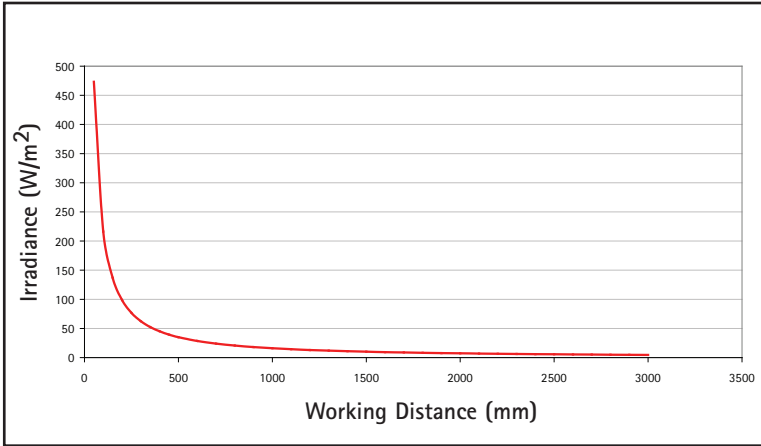
Figure 3 - Irradiance vs. working distance for SF1-870.
